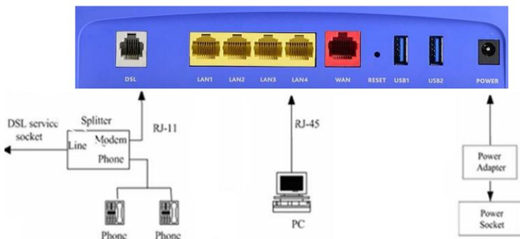
Figure 4 Connecting the DSL router
